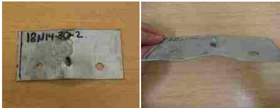
Figure 3.14 Typical Normal-Ductility Flat Sheet after Testing
